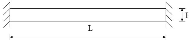
Figure 1. Clamped-clamped beam
