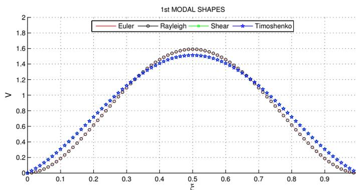
Figure 6. First modal shapes for clamped-clamped beam
