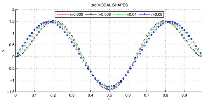
Figure 3. Third modal shapes for clamped-clamped beam
