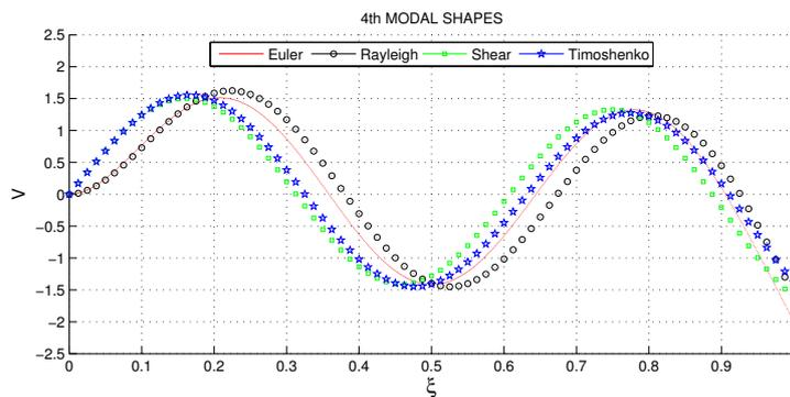
Figure 14. Fourth modal shapes for clamped-free beam
