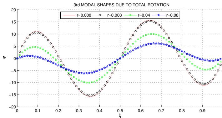
Figure 5. Third modal shapes due to complete rotation
