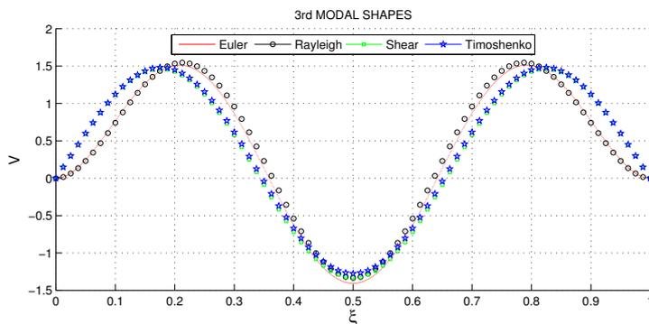
Figure 8. Third modal shapes for clamped-clamped beam
