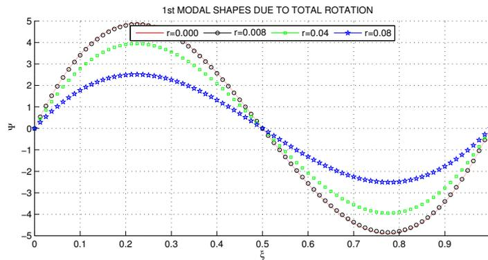
Figure 4. First modal shapes due to complete rotation
