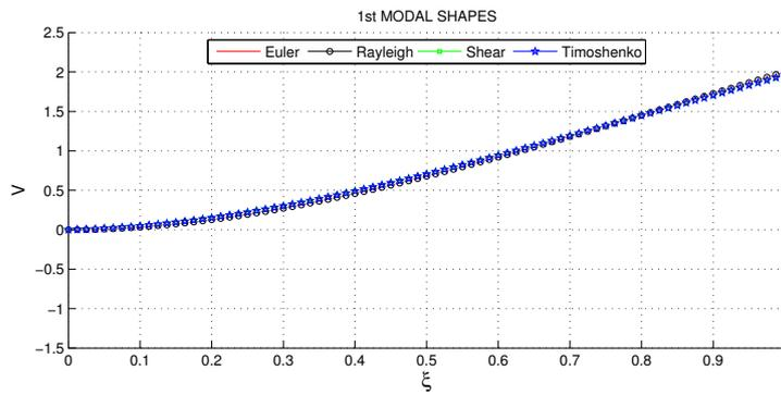
Figure 11. First modal shapes for clamped-free beam
