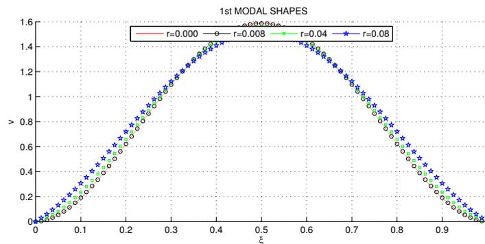
Figure 2. First modal shapes for clamped-clamped beam
