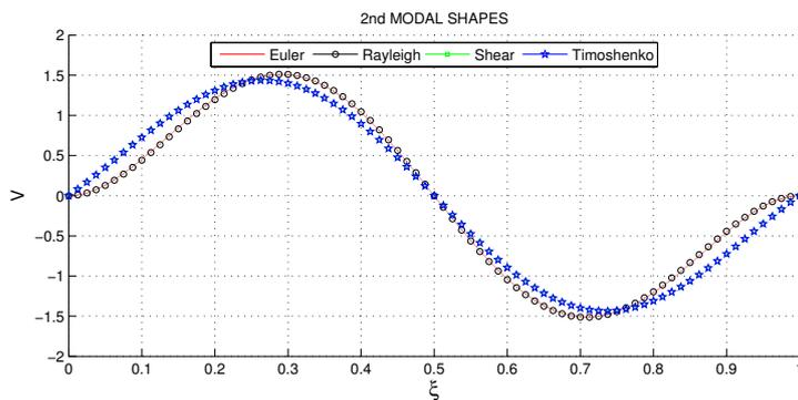
Figure 7. Second modal shapes for clamped-clamped beam
