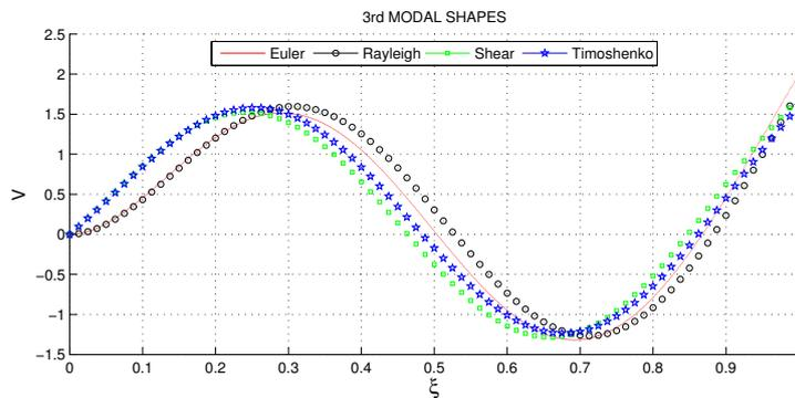
Figure 13. Third modal shapes for clamped-free beam
