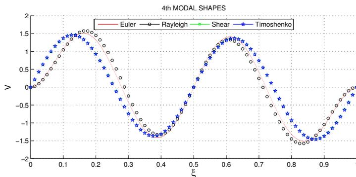
Figure 9. Fourth modal shapes for clamped-clamped beam
